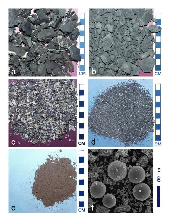
Figure 3. TDF, coal and combustion products from the Purdue University experiment. a) TDF; b) coal; c) bottom ash; d) mechanical collector ash; e) electrostatic precipitator ash (a-e all at same scale); f) scanning electron image of the electrostatic precipitator ash shown in e).
