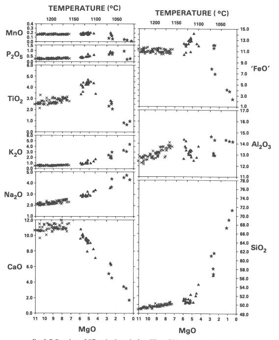
FIG. 8. Bulk analyses of differentiated samples from Kilauea Iki lava lake, plotted against MgO. All quantities in weight percent. Wet chemical analyses of olivine-phyric rock (crosses) and of segregation veins and oozes (triangle) as in Figure 3. Bulk compositions shown by stars were obtained by microprobe analyses of fused glasses and/or by rastered-beam analyses of the differentiated veinlets in polished section. Where both methods were used they gave comparable results.
