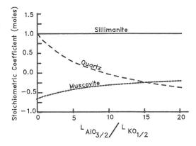
FIG. 4. The stoichiometry of the overall reaction within the sillimanite segregation as a function of the ratio of the aluminum and potassium diffusion coefficients. The stoichiometry given for this reaction in the text (reaction (A)) was calculated using  $(L_{AIO_{3/2}})/(L_{KO_{1/2}}) = 6$ .
