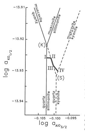
FIG. 8. Activity diagram showing conditions in the model illustrated in Fig. 5. Only selected portions of stable univariant lines (solid) and second-order univariant lines (dashed) are shown. Refer to Fig. 3 for complete diagram. Points I, III and IV correspond to reaction interfaces with the same numbers given in Fig. 5. The kyanite-absent and sillimanite-absent invariant points are labelled (K) and (S), respectively.
