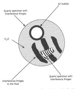
FIG. 5. Typical appearance of a solid sample in liquid water with an air bubble in a circular rhenium gasket hole 500  $\mu$ m in diameter. The portion of the sample illuminated with laser light shows coarse fringes due to interference between light reflected from the two anvil faces. The fine fringes in the solid quartz sample are caused by interference between light reflected from the top and bottom of the platelet.
