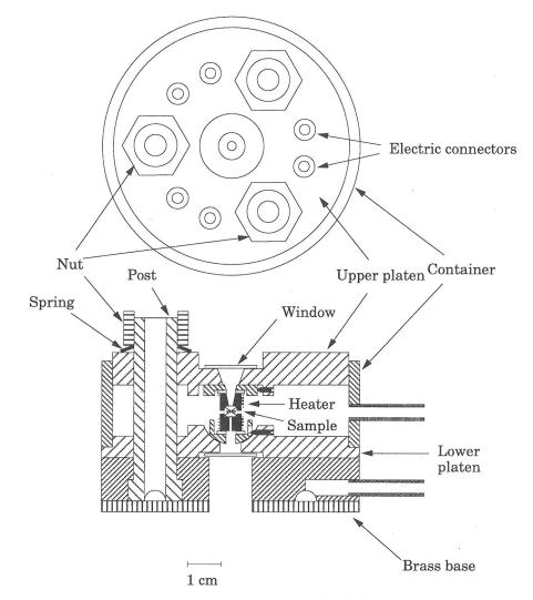
FIG. 1. Plan and elevation of the new diamond anvil cell. The diameter of the cell is 7.62 cm. The height is 5.72 cm. The base is constructed of brass; the platens, posts, and cylinder are constructed of stainless steel.
