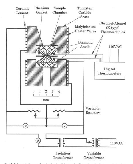
FIG. 2. Schematic diagram showing details of the sample, diamond anvils, heaters, and the electric circuits for heating, controlling, and measuring the temperature of the sample.
