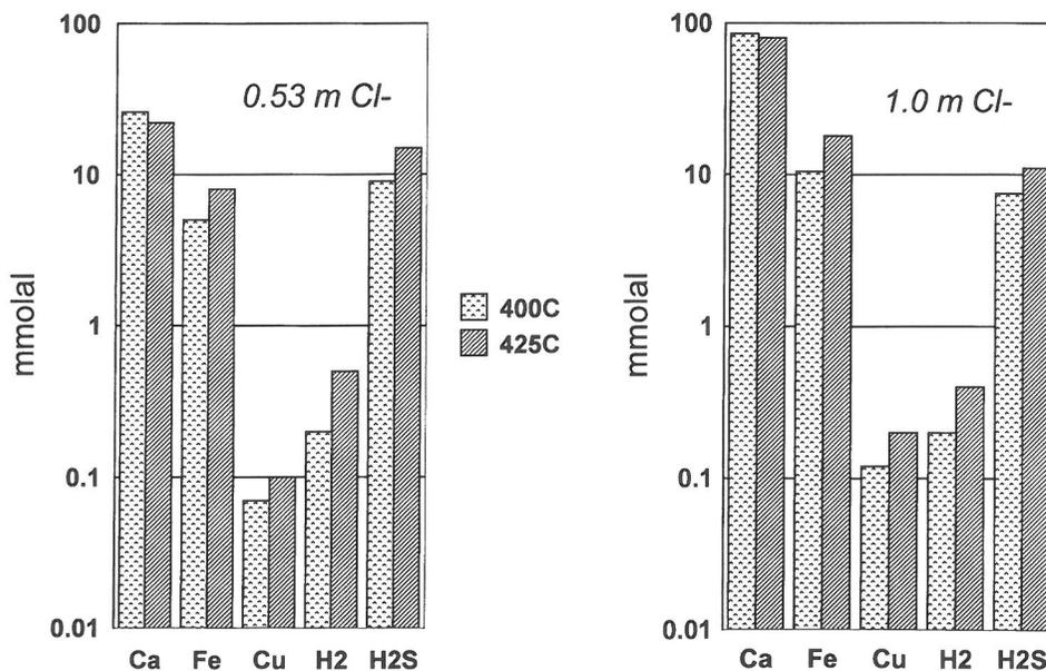
Figure 1. Experimentally determined dissolved Ca, Fe, Cu, H<sub>2</sub>, and H<sub>2</sub>S in 0.53 m Cl<sup>-</sup> (A) and 1.0 m Cl<sup>-</sup> (B) fluid coexisting with plagioclase-epidote-quartz-magnetite-anhydrite-pyrite-chalcopyrite assemblage at 400 and 425 °C, 500 bars.
