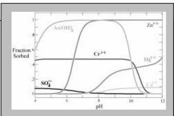
Effect of pH on how metals and other ions sorb onto ferric hydroxide, calculated according to double-layer method.
