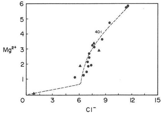
FIG. 13. Calculated evaporation paths for  $Mg^{2+}$  against  $Cl^-$  (in molalities) for brines along the  $Ca^{2+}$ - $Cl^-$  and  $Cl^-$ - $SO_4^{2-}$  chemical divide and the concentrations of these ions in Lake Dabusun (circles) and West Dabusun Lake (triangles) brines. Brine analyses scatter along the calculated 40:1 evaporation path (as do  $Na^+$ ,  $Ca^{2+}$ ,  $HCO_3^-$  and  $SO_4^{2-}$ , not shown), unlike  $K^+$  in Fig. 12.
