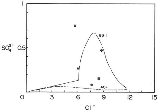
FIG. 9. Calculated evaporation paths for  $\text{SO}_4^{2-}$  against  $\text{Cl}^-$  (in molalities) for the chemical divides bounding the  $\text{Cl}^-$ - $\text{SO}_4^{2-}$  brine field and the concentrations of these ions in the  $\text{Cl}^-$ - $\text{SO}_4^{2-}$  lakes. Tuanjie Lake—diamond, Xiaobie Lake—square, Senie Lake—triangle, Dabiele Lake—circles.
