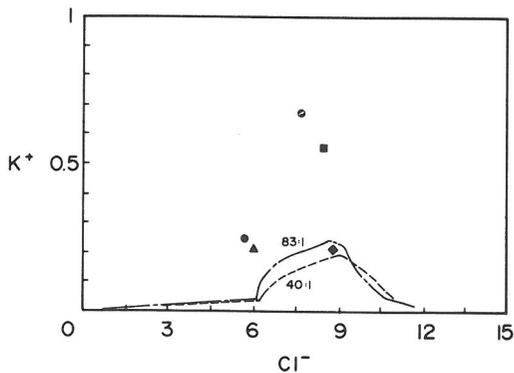
FIG. 11. Calculated evaporation paths for  $\text{K}^+$  against  $\text{Cl}^-$  (in molalities) for the chemical divides bounding the  $\text{Cl}^-$ - $\text{SO}_4^{2-}$  brine field and the concentrations of these ions in the  $\text{Cl}^-$ - $\text{SO}_4^{2-}$  lakes. Tuanjie Lake—diamond, Xiaobie Lake—square, Senie Lake—triangle, Dabiele Lake—circles.
