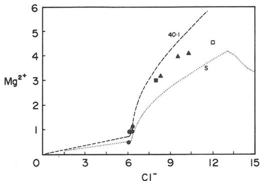
FIG. 7. Calculated evaporation paths for  $\text{Mg}^{2+}$  against  $\text{Cl}^-$  (in molalities) for the chemical divides bounding the  $\text{Ca}^{2+}$ - $\text{Cl}^-$  brine field and the concentrations of these ions in the  $\text{Ca}^{2+}$ - $\text{Cl}^-$  lakes and karst pools. Donglin Lake—open square, Xiezhuo Lake—filled square, North Huobusun Lake—open triangle, karst pools north of Dabusun Lake—filled triangles, karst pools near springs (west of Xiezhuo Lake)—filled circles.
