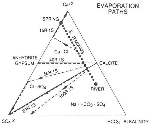
FIG. 3. The compositions of river inflow and spring inflow mixtures lie along the line S-R mixing. Evaporation paths for river waters, spring waters and several mixtures (by weight) of river inflow and spring inflow (including the mixtures for chemical divides in Fig. 2) are shown. Evaporation paths calculated using the thermochemical model of HARVIE *et al.* (1984).
