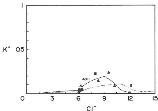
FIG. 8. Calculated evaporation paths for  $\text{K}^+$  against  $\text{Cl}^-$  (in molalities) for the chemical divides bounding the  $\text{Ca}^{2+}$ - $\text{Cl}^-$  brine field and the concentrations of these ions in the  $\text{Ca}^{2+}$ - $\text{Cl}^-$  lakes and karst pools. Donglin Lake—open square, Xiezhuo Lake—filled square, North Huobusun Lake—open triangle, karst pools north of Dabusun Lake—filled triangles, karst pools near springs (west of Xiezhuo Lake)—filled circles.
