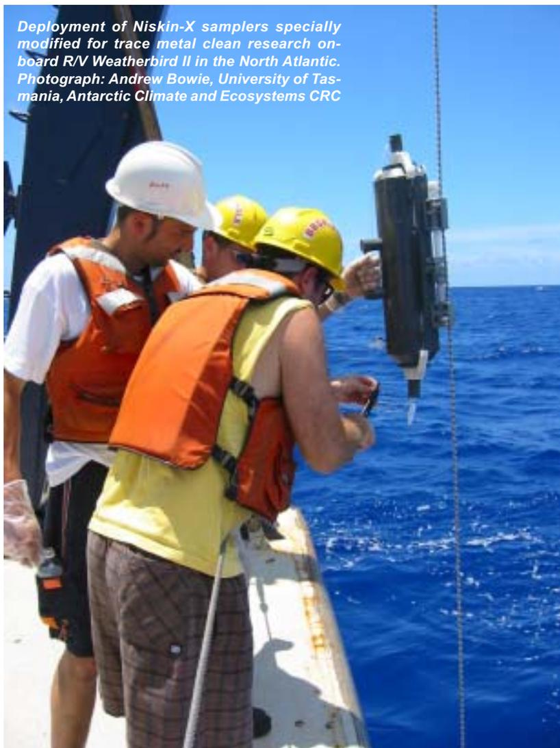
*Deployment of Niskin-X samplers specially modified for trace metal clean research on-board R/V Weatherbird II in the North Atlantic. Photograph: Andrew Bowie, University of Tasmania, Antarctic Climate and Ecosystems CRC*
