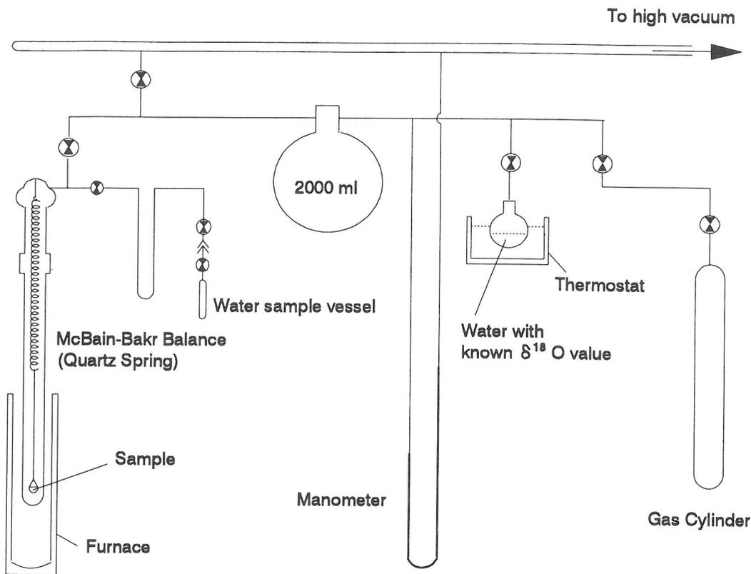
FIG. 1. McBain-Bakr balance used for thermogravimetric studies of zeolites at controlled temperature and  $P_{\text{H}_2\text{O}}$ , studies of gas absorption by zeolites, and extraction of channel water from zeolites.
