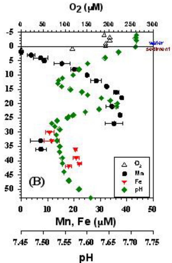
**Figure 3.** (A) Distribution of dissolved  $O_2$ , Mn and Fe in porewaters from Raritan Bay New Jersey.  $O_2$  and Mn do not overlap and the agreement between the voltammetric sensor and the Clark  $O_2$  sensor is excellent. (B) Profile with pH data from C. Reimers.  $O_2$  is not detected at 2 mm depth and Mn is first detected at 3 mm. The maximum in pH occurs with the  $Mn^{2+}$  maximum. (C) ROV ready to deploy the electrodes.
