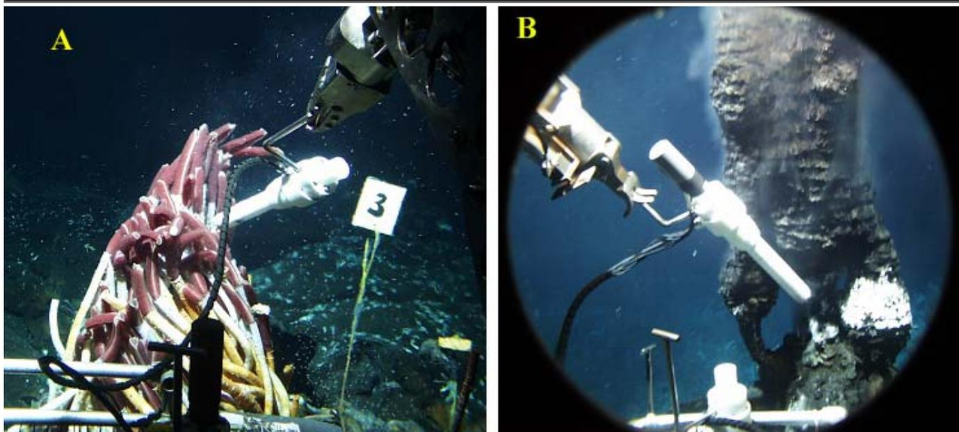
**Figure 5.** Deployment of electrodes near (A) *Riftia pachyptila* and (B) a beehive vent structure.
