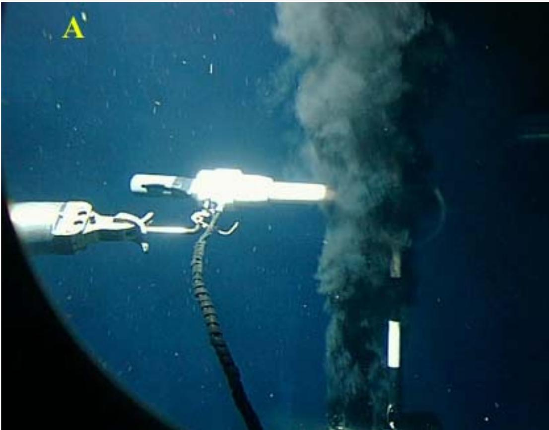
**Left: Figure 4. (A)** Positioning of the electrodes 0.5 m above a black smoker chimney.
