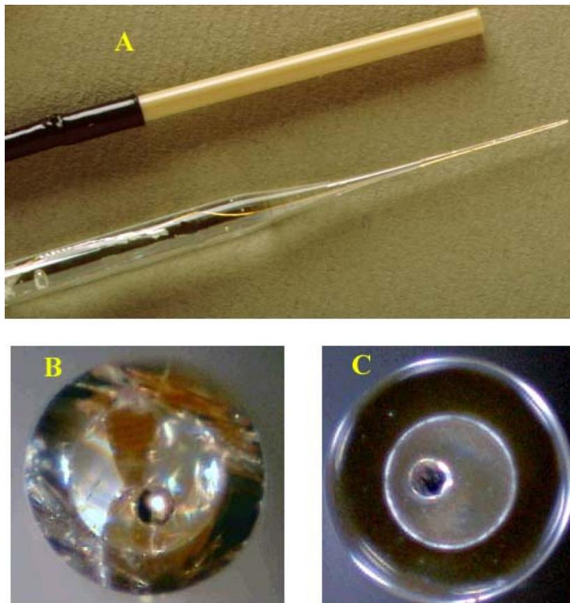
**Figure 1.** (A) A glass encased and PEEK electrode – the Au wire is soldered to the conductor wire and fixed with a non-conductive epoxy. (B) The tip of a 100 mm diameter Au electrode in glass after initial construction but before sanding and polishing. (C) After final polishing with 0.25 mm polish and prior to plating with Hg solution.
