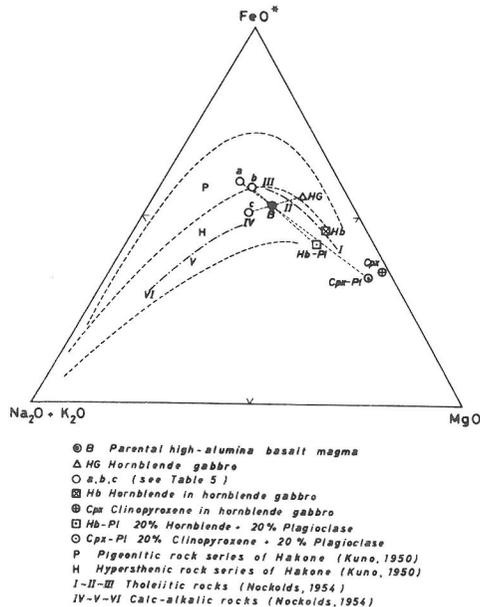
FIG. 5. High-alumina basalt, hornblende gabbro, hornblende, clinopyroxene and residual compositions (from Table 1).
