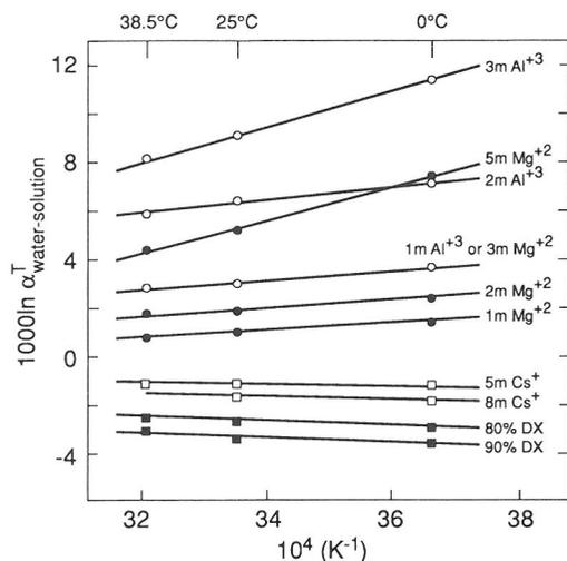
FIG. 3. Temperature dependence of the per mil fractionations between pure water and various solutions. Note the similarity in slopes of structure makers and structure breakers and that the curves for 1 m  $\text{Al}^{+3}$  and 3 m  $\text{Mg}^{+2}$  are identical. At certain critical concentrations of  $\text{Al}^{+3}$  and  $\text{Mg}^{+2}$ , the slope of the curves change, signalling a transition to another structural state of the solution.
