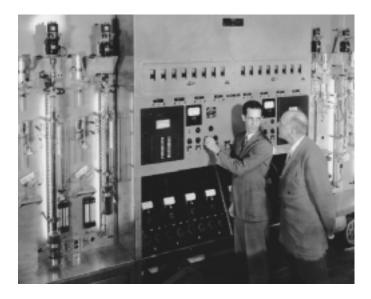
John, the analytical chemist, demonstrating laboratory-scale petroleum distillation unit at Whiting laboratory.
