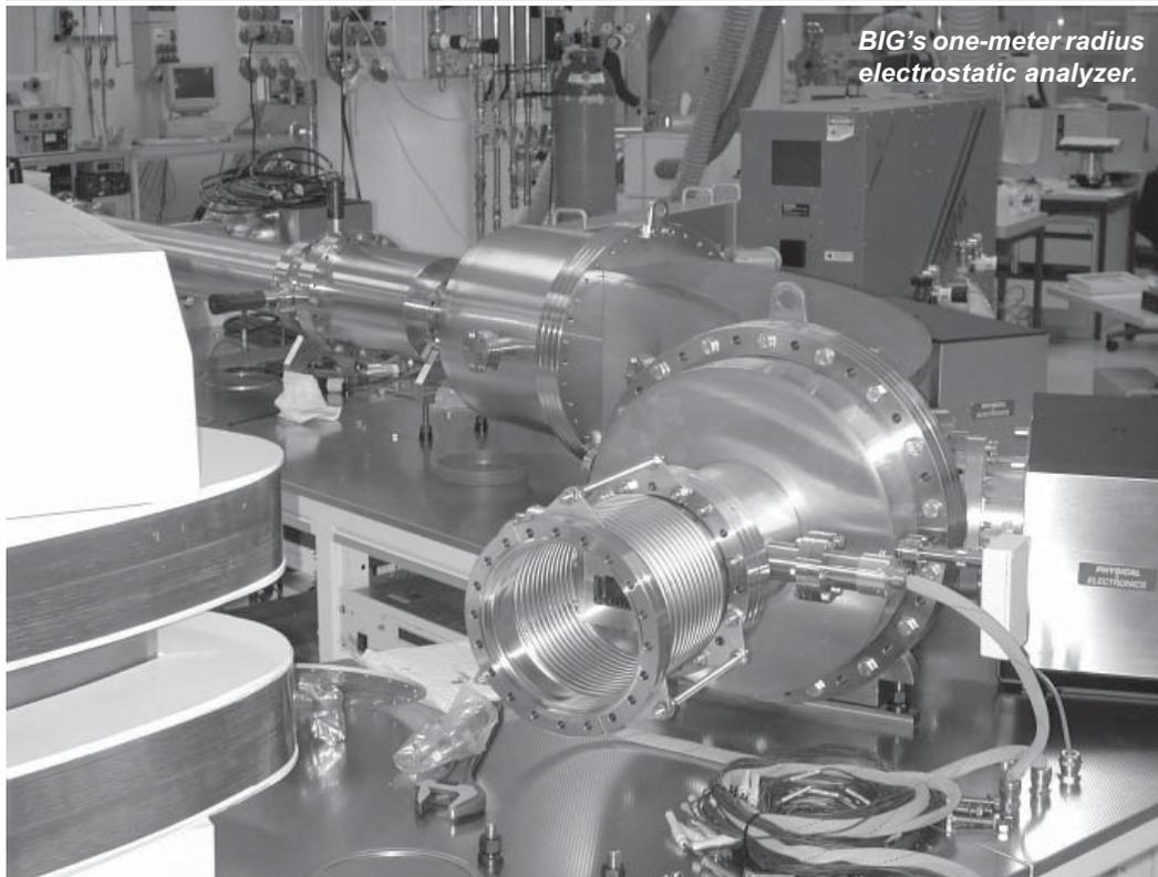
*BIG's one-meter radius electrostatic analyzer.*
