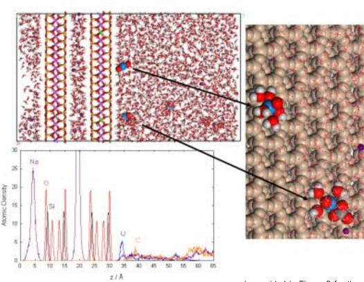
the Schrodinger's equation is solved for every dynamics time step, although simulation time is limited on the order of several picoseconds.
