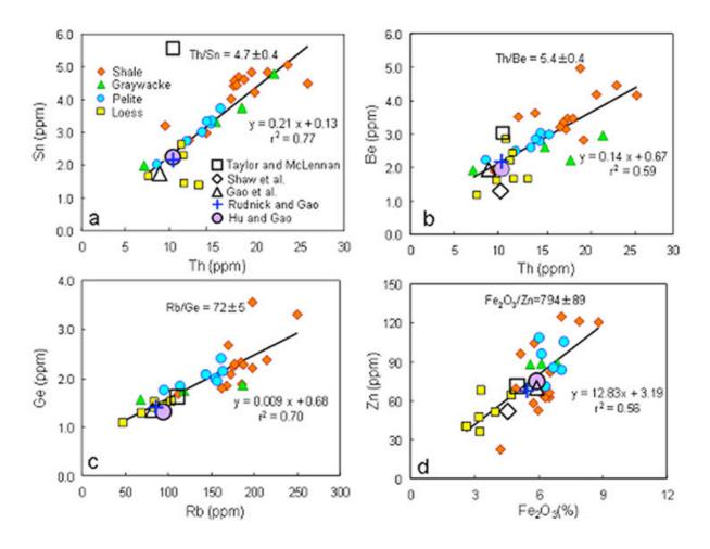
**Figure 2.** Examples of correlations between elements in various fine-grained clastic sedimentary rocks and loess (Hu and Gao, 2008): (a) Th-Sn, (b)Th-Be, (c) Rb-Ge, and (d)  $Fe_2O_3$ -Zn. Lines represent linear fit to data. r is correlation coefficient. Superimposed are upper crustal composition estimates of Taylor and McLennan (1985, 2009), Shaw et al. (1986), Gao et al. (1998b), Rudnick and Gao (2003), and Hu and Gao (2008).
