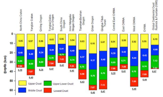
**Figure 4.** Average crustal structure for different tectonic units in China. All velocities are reported at 600 MPa and room temperature (Gao et al., 1998a). The underlined number below each column indicates average Vp for the total crust.
