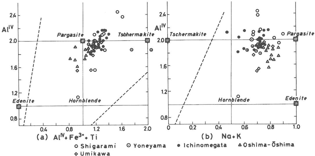
FIG. 3. Hornblende compositions in Al<sup>IV</sup>-(Al<sup>VI</sup> + Fe<sup>3+</sup> + Ti) and Al<sup>IV</sup>-(Na + K) diagrams. Data from TAKESHITA (1975), AOKI (1971), YAMAZAKI *et al.* (1966), SHIMAZU *et al.* (1979), ONUKI (1965), YAMAMOTO (1984). Symbols as in Figure 4.
